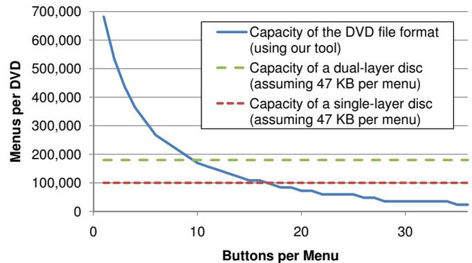
Fig. 2. The number of menus that can fit on a DVD is constrained by both the DVD file format as well as the physical capacity of the disc. Our tool allows many menus to be represented within the DVD file format; the capacity of the format depends on the number of buttons (options) per menu. For the applications in this paper, we are ultimately constrained by the physical capacity of the disc.
